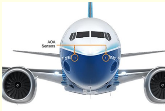
Picture 4 - the position of AOA Sensors (source: www.boeing.com )
